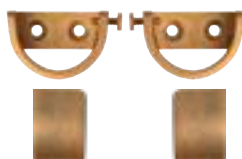
IM125 1 1/4" steel inside mount brackets 1 1/8"H x 1 3/8"W backplate, 3/4"Deep, 1/8" thick backplate per bracket (sold in pairs)
