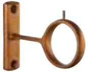
EB1 steel eyelet bracket, single 3½" return, 1"W x 3½"L backplate, eyelet 1"ID
